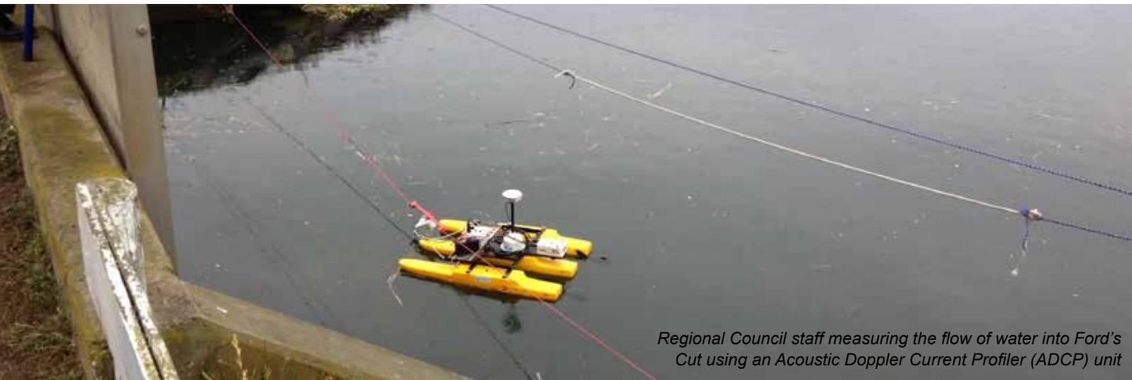
*Regional Council staff measuring the flow of water into Ford's Cut using an Acoustic Doppler Current Profiler (ADCP) unit*
